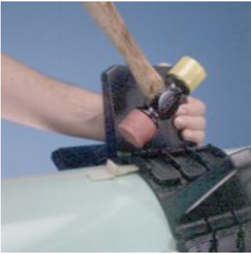
7A. To tighten Ranger II securely to carrier pipe, back Slide-Lock completely out of the slot. If needed, push segments together by hand.
