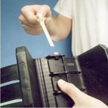
7A. To tighten Ranger II securely to carrier pipe, back Slide-Lock completely out of the slot. If needed, push segments together by hand.
