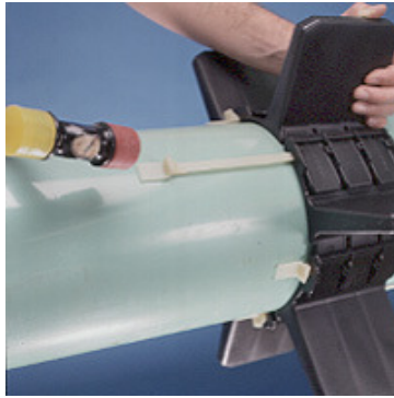
7B. Re-insert Slide-Locks completely into segment by lightly tapping Slide-Lock back into position while holding the Slide-Lock against pipe.
