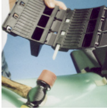
B) Remove Slide-Lock by backing it out, do not pull it through to remove the broken piece. Tap broken piece back out.
