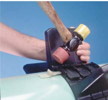
7A. To tighten Ranger II casing spacer, back the Slide-Lock completely out of slot and, if needed, push segments together by hand. Ratchet the Slide-Lock in and out to apply tension as the casing spacer assembly tightens down on the pipe.
