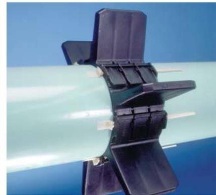
8. Continue steps 7A and 7B until Ranger II Casing Spacer is secure against carrier pipe making certain segment engagement is uniform.
