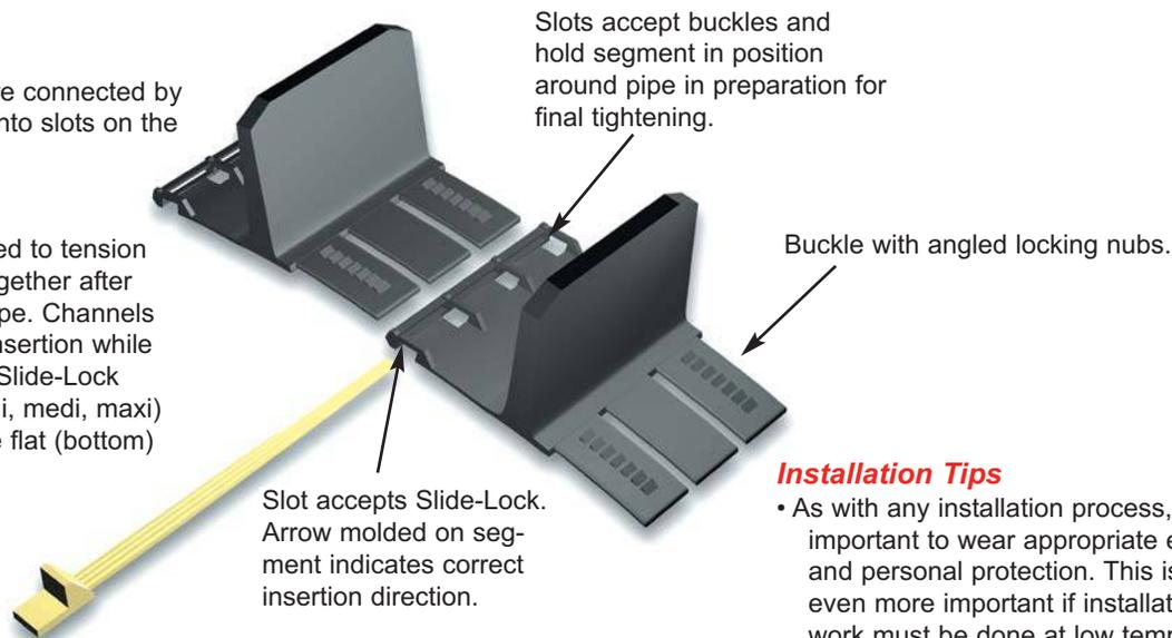
Slots accept buckles and hold segment in position around pipe in preparation for final tightening.
