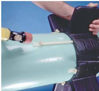
7B. Re-insert Slide-Locks completely into segment by lightly tapping Slide-Lock back into position. **Note:** Make sure buckles are uniformly aligned and inserted into slots.
