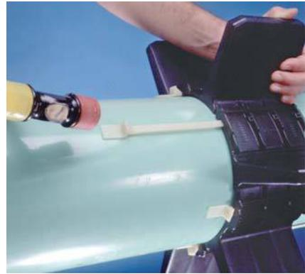
6. Insert all Slide-Locks as far as possible by hand. Complete tightening by lightly tapping each Slide-Lock with a light rubber headed hammer.
