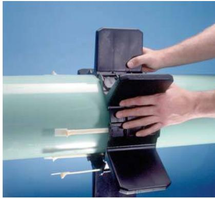
5. Align the buckles and lock into place. Take the final Slide-Lock and slide completely into place. **Note:** Make sure buckles are uniformly aligned and inserted into slots.
