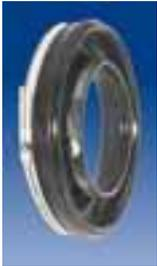
Model "S" standard pull-on end seals are flexible and easily installed on customer specified casing/carrier pipe combinations. Manufactured from 1/8" thick synthetic rubber, Model "S" end seals are extremely robust, resistant to wide variations in environmental conditions while eliminating the possibility of foreign material entering the opening between carrier and casing
