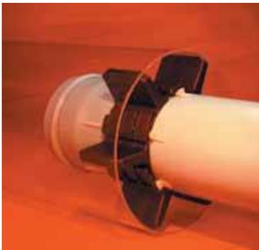
The Ranger II® is a completely non-metallic casing isolator/spacer system that uses molded segments to encircle the carrier pipe. Each segment includes at least one molded-in runner and one slide lock. Customers may choose from any one of five different size bands to allow correct sizing for carrier pipe O.D. ranges from 0.83" up to 37.60" in diameter.
