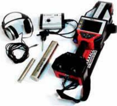
Pig Tracking Equipment plays an essential role in an operator's pigging activities. Knowing where the pig is and finding it if it gets stuck can save the user costly down time and frustration. Drinkwater Products keeps a wide range of tracking equipment for rental or purchase and has the hands-on experience to help you with product selection and tracking strategy.
