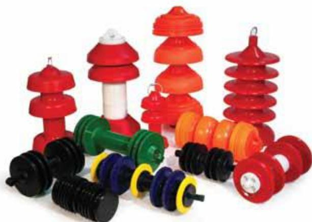
Cast-Urethane pigs are rugged, versatile pigs that can be used for a number of applications including batching, cleaning and dewatering. Cast-Urethane pigs can be run multiple times and are generally more aggressive than foam pigs.
