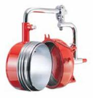
Over 60 years of reliable field service has made Yale closures the leader in the industry. With the original Figure 500 closure, we were the first to develop the inherent safety and operating ease of a threaded closure. The Figure 500 closure design combines simplicity and reliability through the use of a rugged, modified ACME thread to fasten the cap to the hub. The pressure seal is achieved by an O-ring set in the face of the hub. Figure 500 closures are manufactured in sizes 2"-54".
