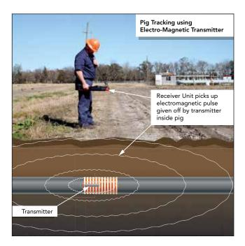
Electromagnetic Transmitters give off a pulse which is picked up by a receiver unit. This allows the operator to track a moving pig or locate a stuck pig.
