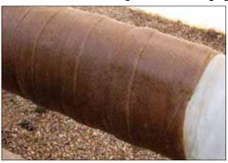
Trenton HT-3000 Wax-Tape® is a specially formulated wax-based tape used for corrosion protection of metal pipe and fixtures experiencing higher than normal temperatures. HT-3000 Wax-Tape can be applied and will perform effectively at continuous operating temperatures of up to **230°F (110°C)** and is designed for use in aboveground and belowground applications.
